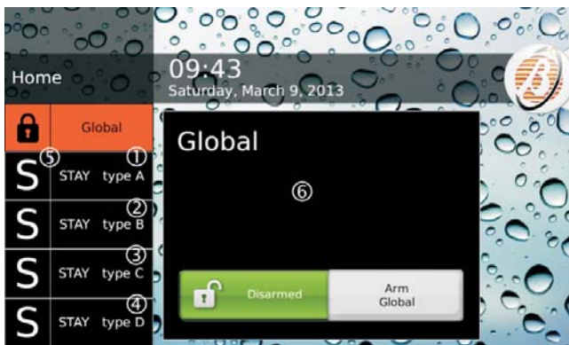
Figure 23 Arming by the Touch Keypad: labels 1, 2, 3 and 4 can be customised, as explained in the text; the corresponding Special arming initial letter will be put in position 5; the description assigned to the arming selected will appear in window 6, as explained in the text.
